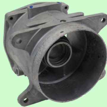
Excessive pitting, interior & exterior
