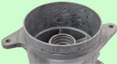
Excessive pitting, interior & exterior
