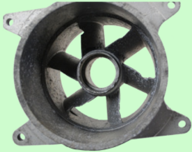
Broken blades, pitted interior & exterior
