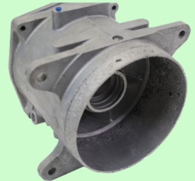
Excessive pitting, interior & exterior
